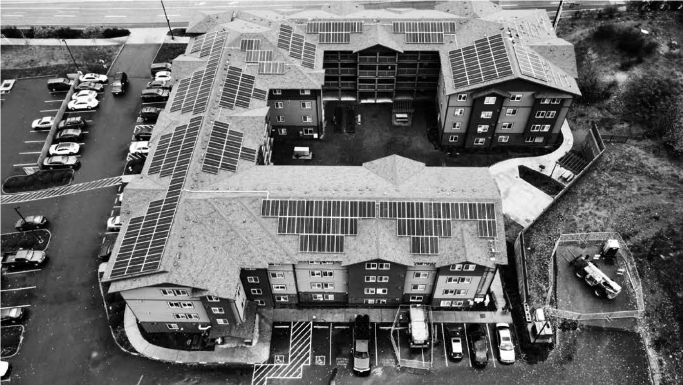
The solar installation at Merritt Manor, a low-income housing development with 82 apartments in East Olympia, has 324 solar panels and will produce about 129 megawatt hours of electricity a year - roughly a third of the building’s total consumption. With the panels, every apartment will save about $260 dollars a year on energy. Installation by South Sound Solar.
